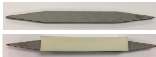
Figure 4-2: Picture of the FDM-fabricated dielectric rod waveguide without the cladding (top) and with the ABS cladding (bottom).
